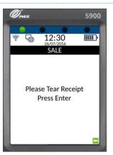
Tear off the receipt (after printing has completed) from the axept<sup>®</sup> S900 terminal and press the key on the keypad to continue.
