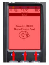
Position the (contactless enabled) card or device around the screen area of the terminal for a few seconds until a 'beep' sound confirms the card has been read (the green contactless LEDs will incrementally light up as the card is being read).
