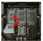
Place the new SIM card in the slot making sure the contacts of the terminal match the contacts of the SIM (the contacts of the sim should be at the base facing away from you) and close the latch.
