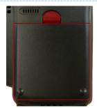
To insert the battery, turn the axept® S900 terminal over so the battery cover latch is visible.
