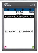
axept® S900 supports Dynamic Host Configuration Protocol (DHCP) which automatically obtains all network settings.
