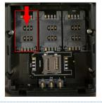
Slide in the direction indicated to open the SIM card latch and place the SIM card in the slot making sure the contacts of the terminal match the contacts of the SIM.
