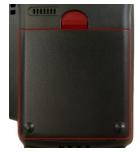
To insert or replace the SIM card in the terminal, turn the axept® \$900 terminal over so the battery cover latch is visible.
