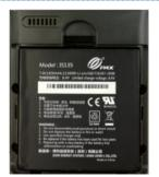
Once the battery is in place, clip the battery cover back onto the terminal.
