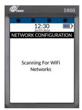
If the option to manually configure Wi-Fi was not selected, axept® \$900 will start to scan for available Wi-Fi networks.
