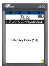
If the network security type selected is '**WEP**', enter the key index value (this step is not required if other network security types are used).
