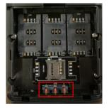
Place the battery into the battery compartment making sure the contact points of the battery align with the connectors of the terminal (as highlighted).
