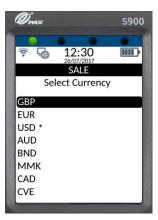
Use the navigation keys ( and on the keypad to highlight the required currency and press the key on the keypad to confirm.
