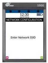
If the option to manually configure the network settings was selected, the SSID for the network will be required. Enter the SSID using the terminal's keypad.
