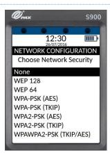
Use the and keys on the keypad to highlight the network security type required.
