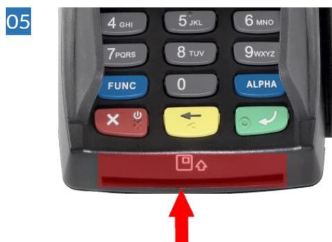
Insert the card (with the Chip of the card on top, facing towards you) into the Chip and PIN card slot at the base of the terminal.
