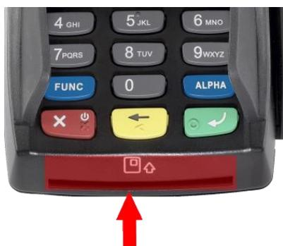
Alternatively, ask the cardholder to insert their card into (with the Chip of the card on top, facing towards you) into the Chip and PIN card slot at the base of the terminal.
