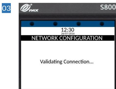
**axept**® S800 validates the network connection and communicates with the DHCP server to obtain an IP address and other network settings.
