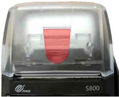
Insert the thermal paper roll into the axept® S800 terminal.
