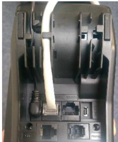
Once connected, run the cables through the cable management sections of the axept® S800 (as shown left).
