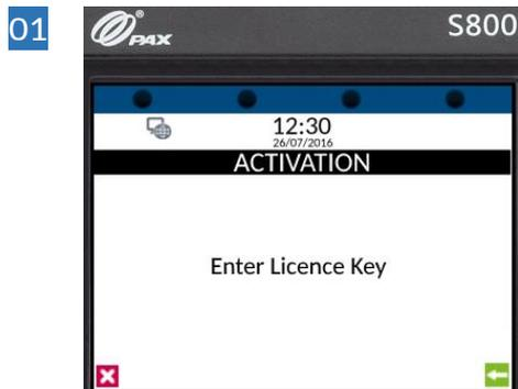
Using the keypad, enter the Licence Key sent to you by Optomany (to use alpha characters, press the numeric key containing the alpha character required multiple times until it is displayed).
